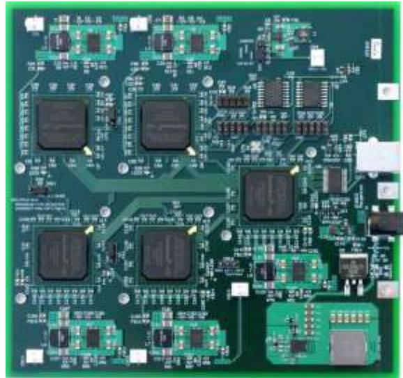
**Fig. 8** PRD 8 PCB – 819.2 GHz. Shown without heat sinks.
